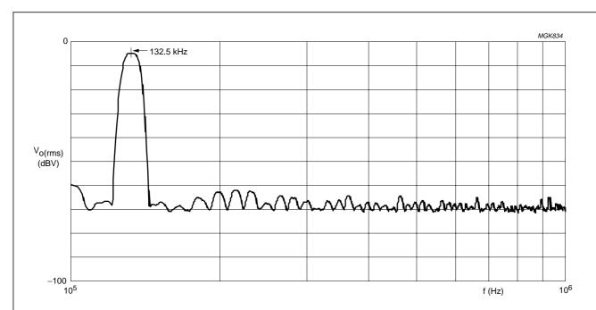
Resolution bandwidth = 9 kHz; top: 0 dBV (RMS) = 120 dB $\mu$ V (RMS); marker at –5 dBV (RMS) = 115 dB $\mu$ V (RMS); the CISPR16 network provides an attenuation of 6 dB, so the signal amplitude is 121 dB $\mu$ V (RMS).
